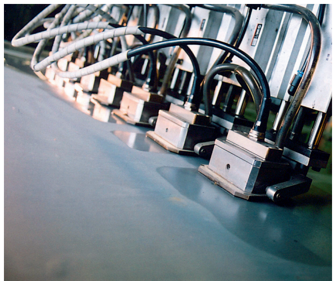
Fig. 2.3_3: Ultrasonic testing already during goods inwards inspection
