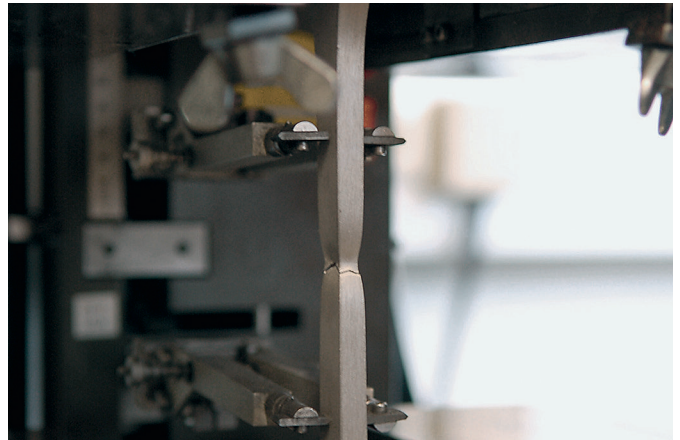
Fig. 2.3_2: Tensile test as one possible destructive test
